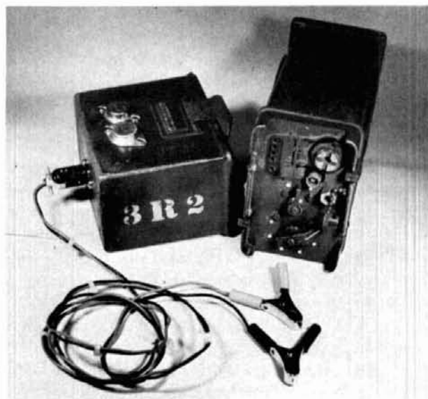
fig. 6. The complete radio set, shown with power supply and cable, measures 3 × 4.75 × 10.34 inches (7.62 × 12.07 × 26.26 cm).
